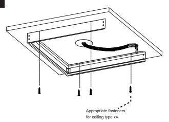
Choose the opening part as close as possible to the junction box prior to securing the surface mount frame to the ceiling. Enaure the frame is square,then slide horizontally till the end of slots prior to fully securing the frame to the ceiling.
