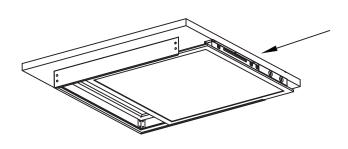
Put the wire conduit hose as close as possible to the surface mount opening before placing/inserting the luminaire into it partially. Make all electrical connections according to local code and make sure wire conduit hose is long enough for wiring connection job.
