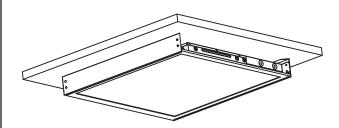
Push the conduit hose back into the surface mount frame properly ,insert the luminaire fully into the frame. When installed properly, the luminaire will rest on the flanges of the surface mount frames. If the luminaire is not resting properly on the flanges, lift it up and shift it until it rests into place.
