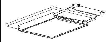
Place the last frame into the slots, Fix the side frame by screw. make sure it get locked tightly, join the last frame to the rested frames by fastening them together with appropriate fasteners.
