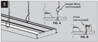
Secure the Flange Kit to the building structure by Hanger Wires(not included) (Fig. A), alternatively screw(not included) to Wood Blocking (Fig. B).
